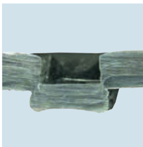
Schliffbild einer dreilagigen Clinchverbindung S-DF / Cross-section of a three-layer connection S-DF
