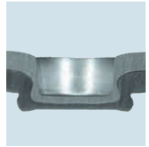
Cross-section of optimised clinching element
