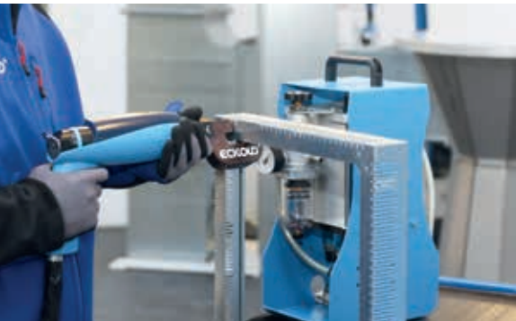
Hand-held portable devices with pneumohydraulic drive
