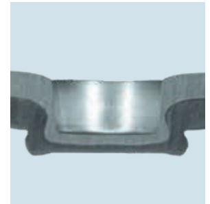
Cross-section of optimised clinching element
